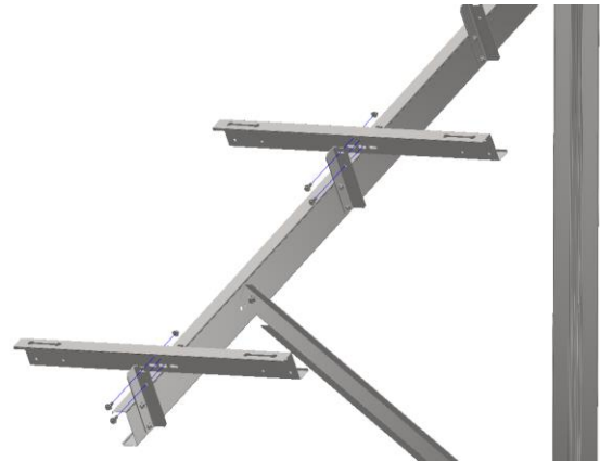
Image 7.1-2 Aligning the Steel Purlins
