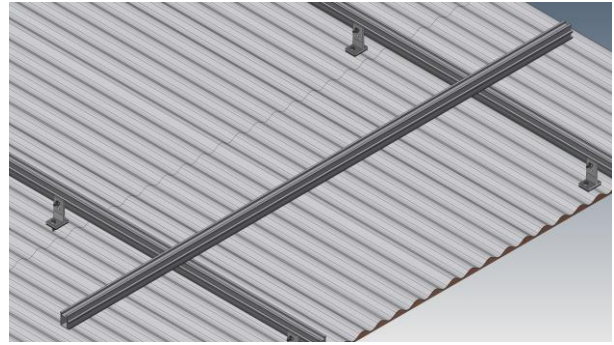
Image 8.1-1 – Upper Rail Perpendicular to the Base Rails
