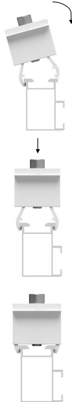
Image 7.1 Module Clamp Installation
